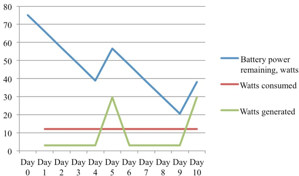
**Figure 3** – Solar recharging chart, Toronto example (Solar panel horizontal)
