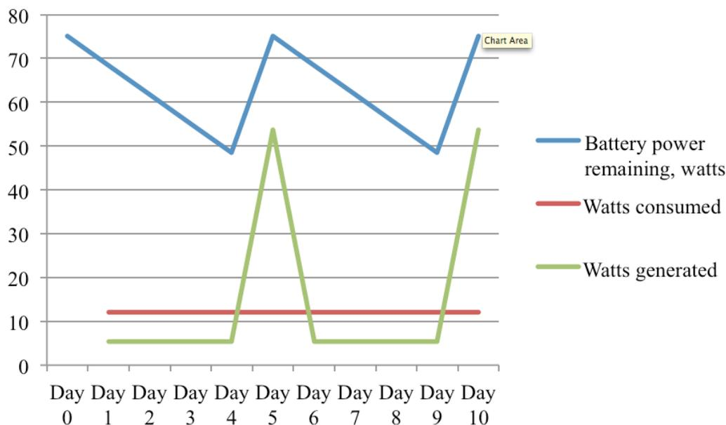
**Figure 4** - Solar recharging chart, Toronto example (Solar panel tilted 31°)
