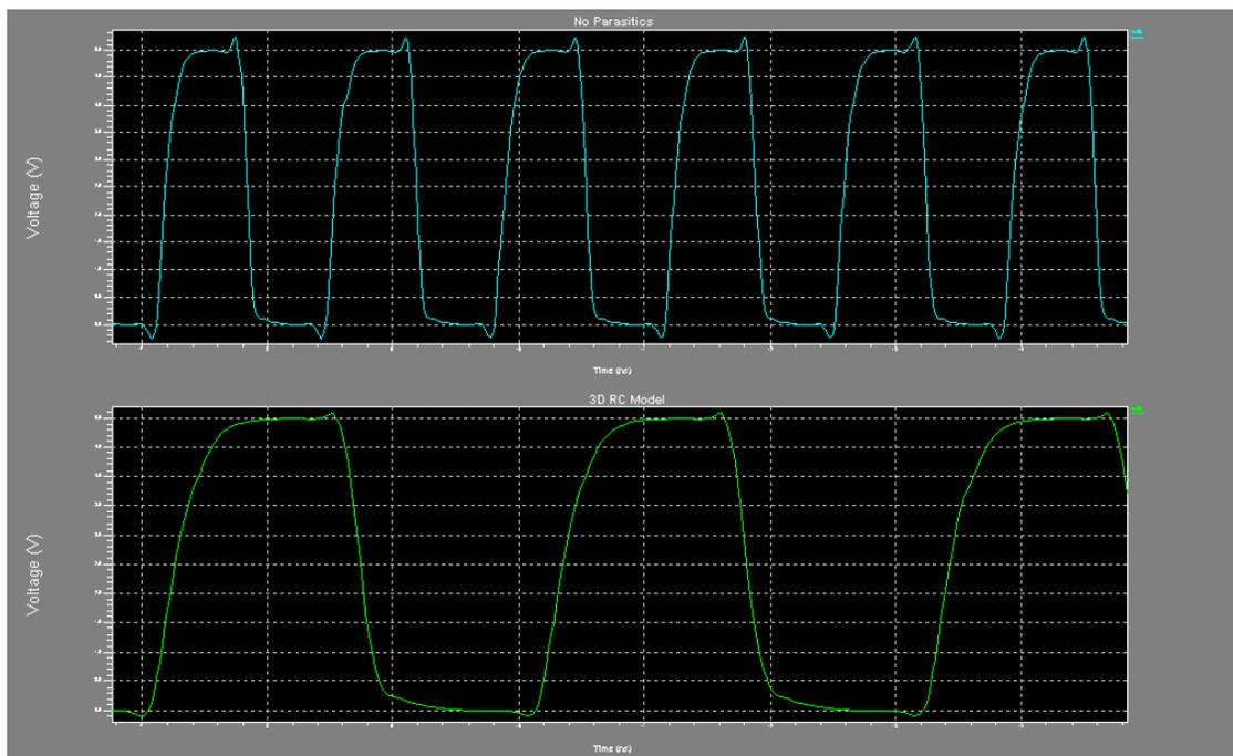
**Figure 6 - Operating Frequencies Before and After Netlist Reduction**
